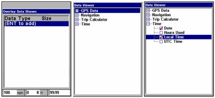
From Overlay Data Shown (left) press ENT to see Data Viewer (center). Select a category and press ENT; then select information to float on screen and press ENT (right).
